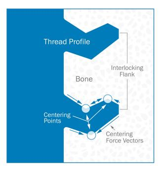
Unique thread geometry instantly and circumferentially interlocks with bone by entrapping and containing bone between the thread form.
