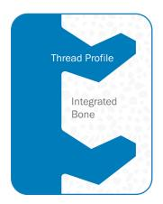
Unique thread geometry instantly and circumferentially interlocks with bone by entrapping and containing bone between the thread form.
